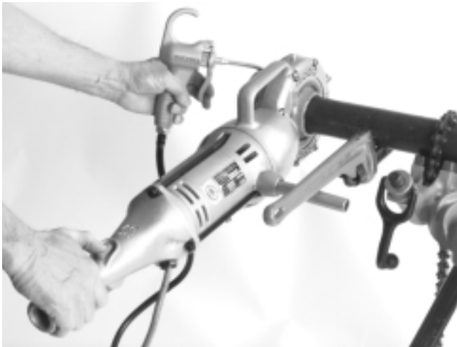
Figure 6 – Threading Using Pipe Wrench As A Support Arm
